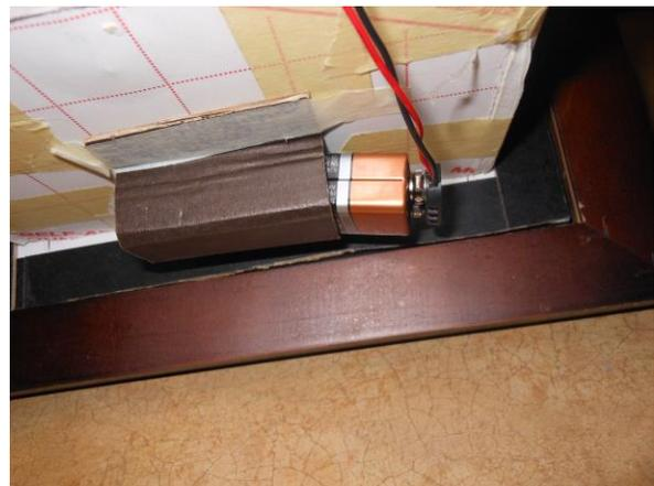
Hook up the battery, and place in the battery cover. Tape all electrical wiring firmly to the outside of the box.
